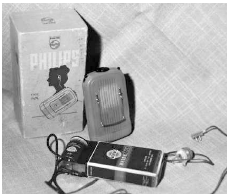
Ill. 11: Small design with subminiature tubes
